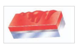
Dry Spray is a rough, textured surface usually confined to a small area that is caused by the paint's lack of ability to flow properly.
