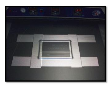
NovAcryl PT Series Photopolymer incorporates a clear PETG base substrate. The PETG is extruded with a UV inhibitor which eliminates light passing through the substrate and exposing the photopolymer in undesired areas.
